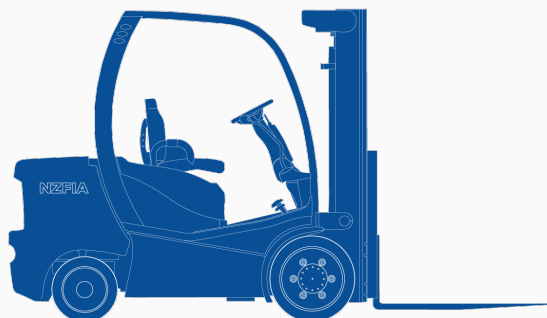
4.1 – Counterbalanced internal combustion engine
